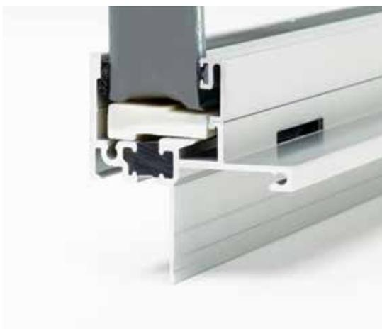
Milgard's Thermal Break Aluminum Windows consist of extruded aluminum, where a "channel" is cut through the aluminum and polyurethane is poured into this channel to separate the interior from exterior extrusion. This process is done to reduce thermal transfer and improve energy efficiency.
